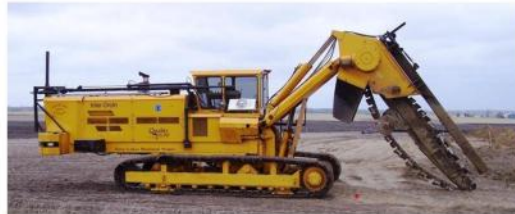
The Inter-Drain chain trencher. Four size choices, mechanical or hydraulic chain drive, vertical and offset available. Cummins, Volvo or Cat power.
